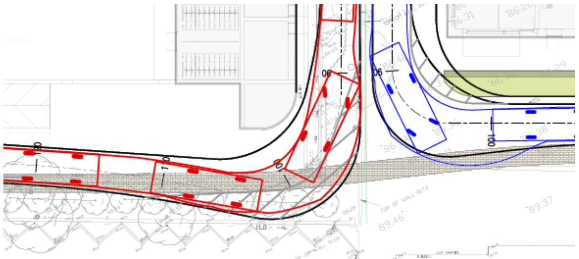
Figure 8 – Swept Path Analyses adjacent to Block A where vehicles are overrunning footways.
