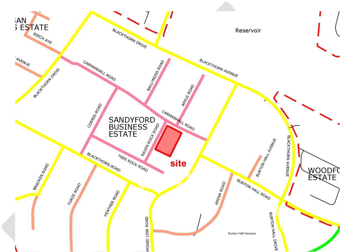
Figure 12 Sandyford Business Estate Road Hierarchy (SUFP Drawing No 7) (Level 1 Roads in yellow and Level 2 Roads in pink)
